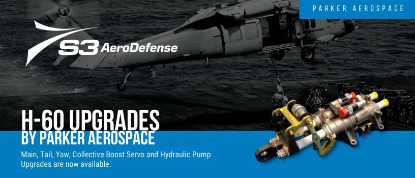
The main focus for improvements is chrome replacement and seal technology improvements to reduce removals for external leakage. Parker, the US Army and Sikorsky identified additional design improvements and incorporated into new design and new dash number configuration.
